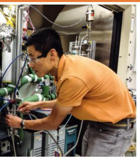
CHILLAX PNNL's Feng Zheng prepares a MOF-filled adsorption heat pump/chiller for testing. In the case of adsorption systems, sending the refrigerant gas from the house to a sorbent positioned outside, and adsorbing (trapping) the gas there, releases unwanted heat to the
