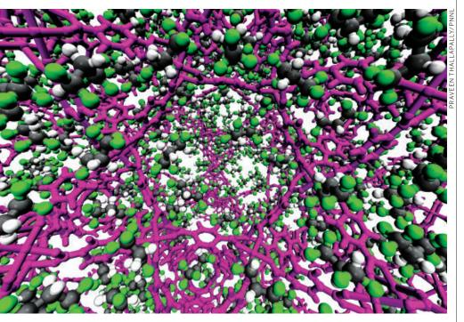
rane to coat the channels with sulfoxide and sulfone groups, and thereby increase the channel hydrophilicity, they soaked up water even when the humidity was as low as 30% (*Energy Environ. Sci.* 2013, DOI: 10.1039/ c3ee40876k).
