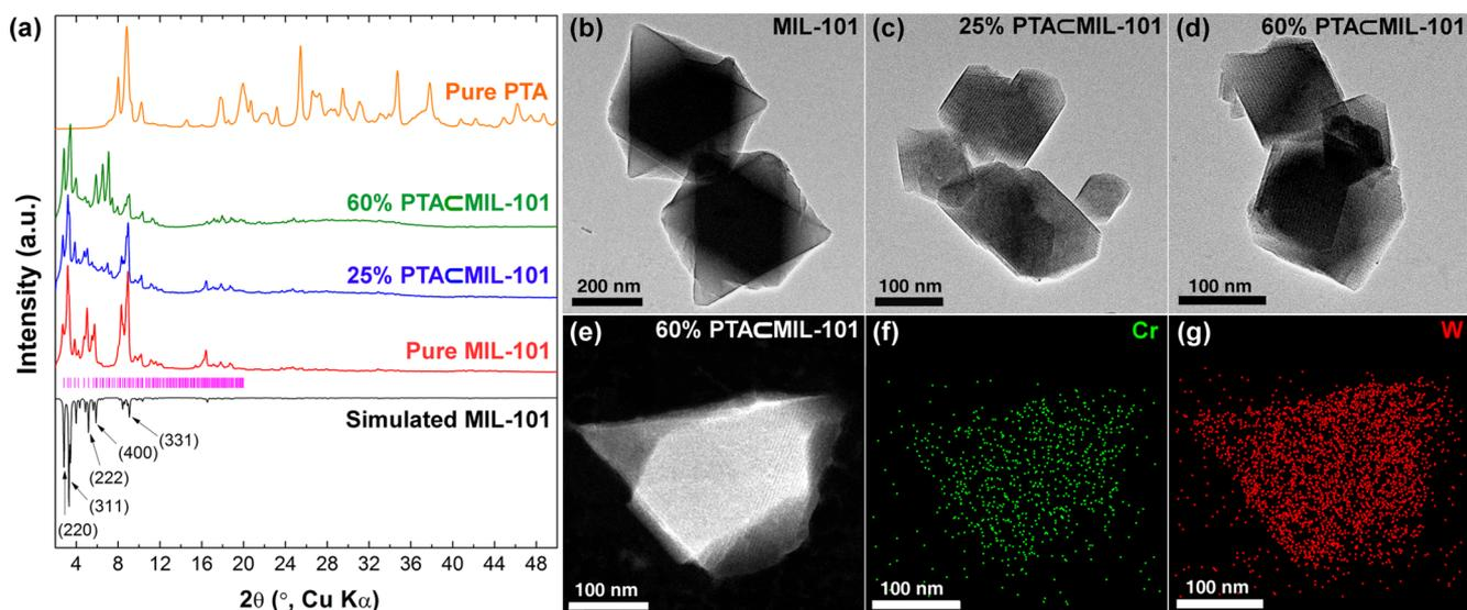
**Figure 1.** Powder XRD patterns for pure PTA, 60% PTACMIL-101, 25% PTACMIL-101, pure MIL-101 and simulated XRD pattern for pure MIL-101 (a). TEM images of pure MIL-101 (b) and MIL-101 that contains 25% (c) and 60% (d) phosphotungstic acid (PTA). Representative HDAAF-STEM image of 60% PTACMIL-101 (e) and corresponding color-coded EDS spectral maps of chromium (Cr) in the framework of MIL-101 represented in green (f) and tungsten (W) in PTA cluster represented in red (g).
