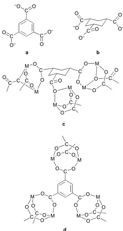
report shows how CTC can be copolymerized with zinc(II) to yield an extended co-ordination solid, formulated as  $Zn_3[(CTC)(C_5H_5N)]_2 \cdot 2(CH_3)_2NC(O)H$ , which possesses channels having a pore diameter of nearly 6 Å.
