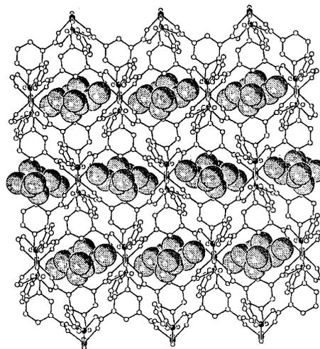
**Fig. 2** The solid-state structure of  $Zn_3[(CTC)(C_5H_5N)]_2 \cdot 2(CH_3)_2NC(O)H$  shown along the *a* axis, where the one-dimensional channels are occupied by dmf (drawn in space-filling style). The hydrogen atoms are omitted and only the zinc atoms are shown as dark spheres with all remaining framework atoms drawn as open spheres
