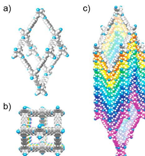
**Figure 1.** Crystal structure of COF-320 obtained by rotating electron diffraction (RED) at 298 K. (a) Adamantane-cage of the diamond net; (b) Representation of the nine-fold interpenetration of the diamond net, viewed along the crystallographic *c*-direction; (c) The square-shaped, one-dimensional (1D) channels running along the *c*-axis.
