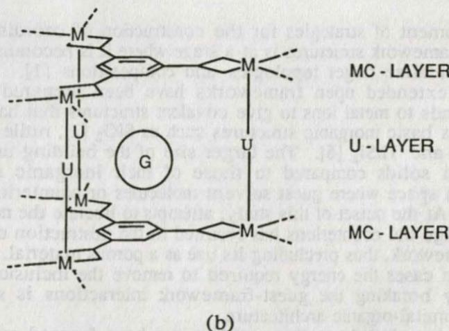
**Figure 1.** (a) The structural formula of 1,3,5-benzenetricarboxylate, and (b) a schematic representation of its coordination to a metal ion to form alternating metal-carboxylate and spacer unit (U) layers leading to voids where guest inclusions (G) reside.
