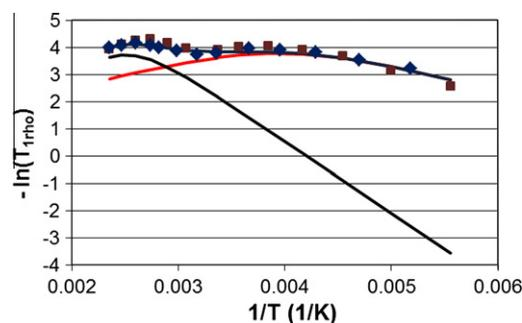
**Fig. 12.** The negative of the logarithm of  $T_{1\rho}$  versus the inverse of the absolute temperature for IRMOF-3 containing  $^{14}\text{N}$  at natural abundance. The experimental points are compared to a simulation, as described in the text ( $\diamond$  – enriched with  $^{15}\text{N}$ ;  $\blacksquare$  – at natural abundance, 99.6%  $^{14}\text{N}$ ). The lines show the predicted temperature dependence of the two contributions to the relaxation.
