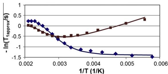
Fig. 4. The negative of the logarithm of the  $^1\text{H}$  spin-lattice relaxation time ( $T_{1\text{approx}}$ ) as a function of the inverse temperature for IRMOF-3 ( $\blacklozenge$  – enriched with  $^{15}\text{N}$ ;  $\blacksquare$  – at natural abundance, 99.6%  $^{14}\text{N}$ ). The solid lines are simulations, as described in the text.
