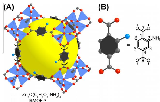
**Fig. 1.** The structure of IRMOF-3 (A). The sphere represents the free volume within the framework. The numerical labeling in (B) is used to note <sup>13</sup>C spectral assignments.
