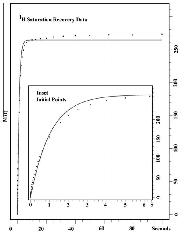
Fig. 3.  $^1\text{H}$  saturation-recovery spin-lattice relaxation data for IRMOF-3 taken at a temperature of 295 K plotted in arbitrary units. The inset shows an expanded view of the initial data points. The smooth line in each is a fit to a single exponential recovery.
