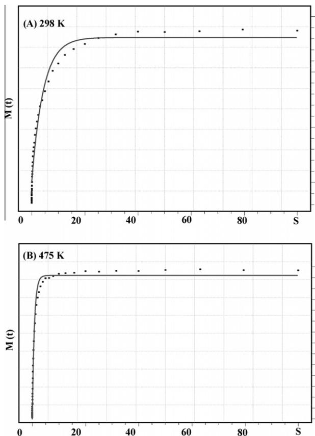
Fig. 5.  $^1\text{H}$  saturation-recovery data for the  $^{15}\text{N}$ -enriched IRMOF-3 at 298 K (A) and at 475 K (B) plotted in arbitrary units. The smooth line in each is a fit to a single-exponential recovery.
