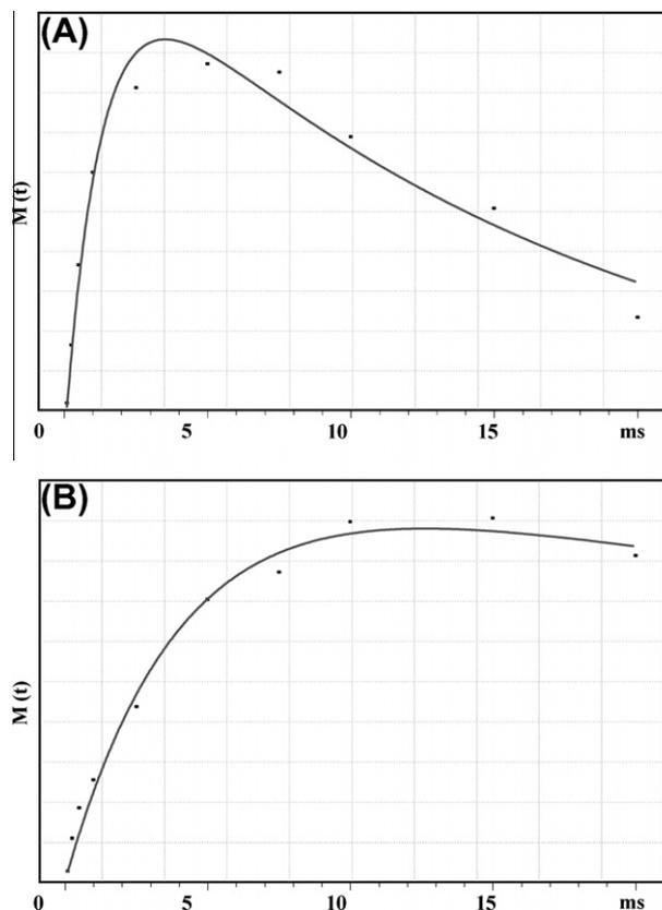
Fig. 9.  $^{13}\text{C}$  CP/MAS variable-contact data (magnetization plotted in arbitrary units) of the carboxyl resonance in a sample of IRMOF-3 containing  $^{14}\text{N}$  at natural abundance (A) and of a sample highly enriched in  $^{15}\text{N}$  (B). The smooth line in each is a fit of Mehring's variable-contact model (see text).
