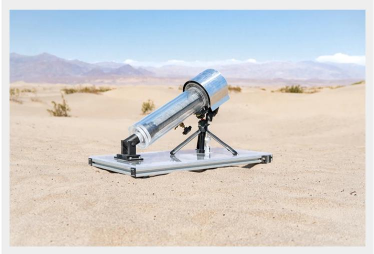
A water harvester containing MOF-303 can collect water from desert air with high efficiency and without power. Credit: Yaghi Laboratory, UC Berkeley
