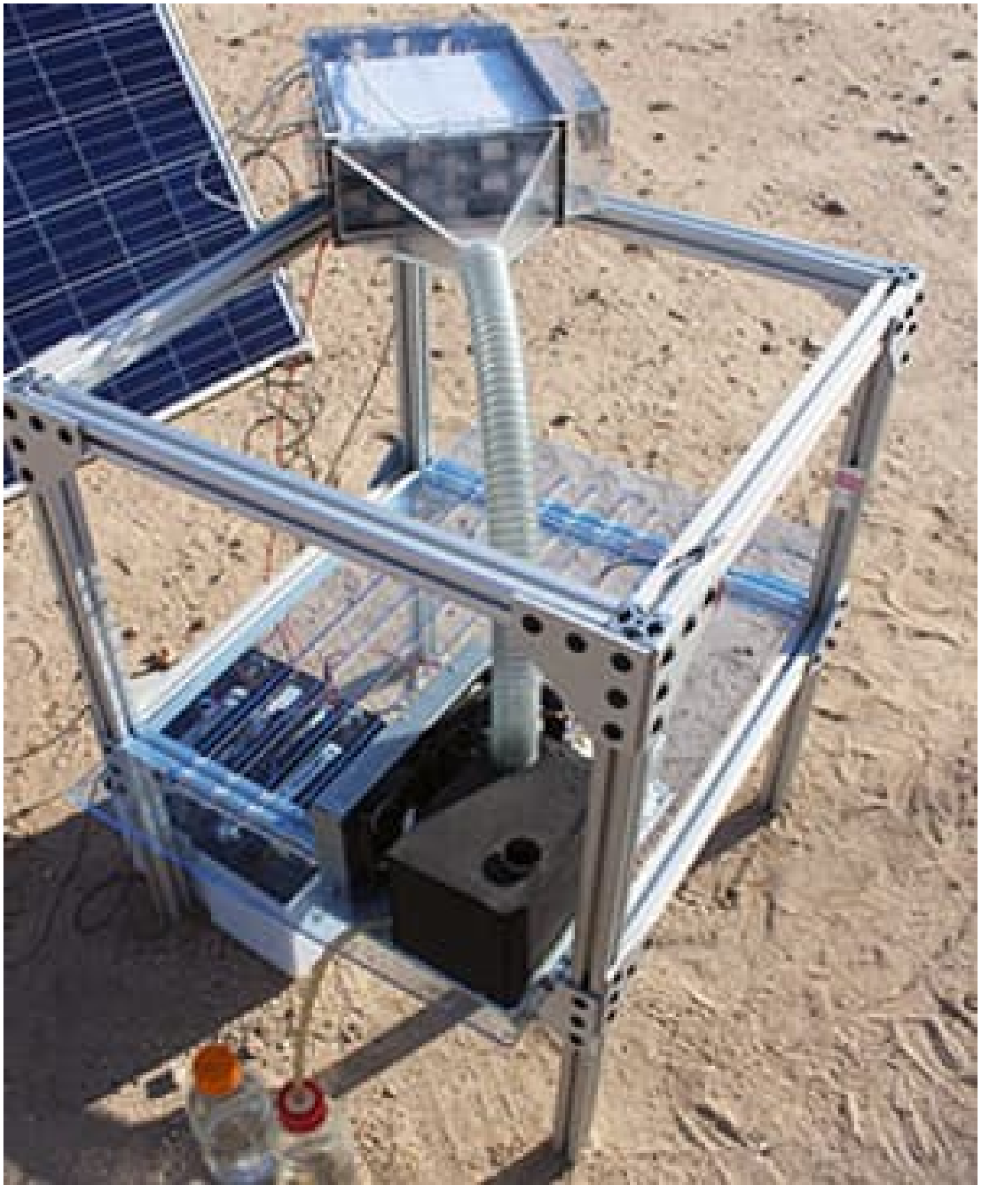
This solar-powered box can harvest over a gallon of water per day.
