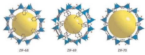
**Carbon traps.** Cagelike zeolitic imidazolate frameworks and their kin excel at straining carbon dioxide out of a mixture of gases, a knack that could lead to CO<sub>2</sub> scrubbers for power-plant smokestacks.
